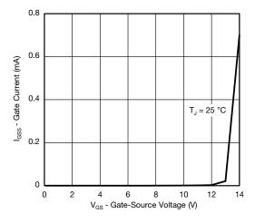
Gate Current vs. Gate-Source Voltage
