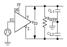
Figure 3: Driver Timing Test Circuit
