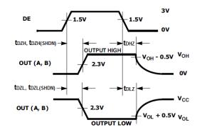
Figure 6: Driver Enable and Disable Times
