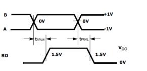
Figure 7: Receiver Propagation Delays
