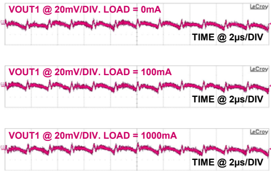
FIGURE 23. PWM1 OUTPUT RIPPLE, MODE = 5V (CCM)
