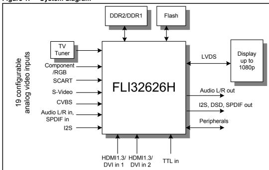
Figure 1. System diagram
