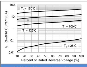
Fig.3 Typical Reverse Characteristics
