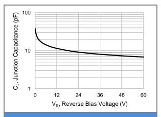
**Fig.2 Typical Junction Capacitance**
