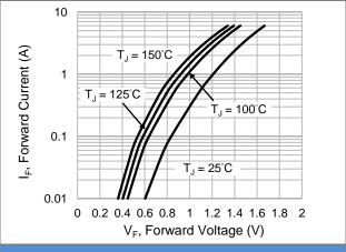
Fig.4 Typical Forward Characteristics
