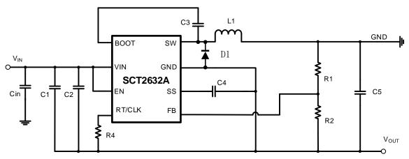
Figure 12. SCT2632A Inverting Power Supply
