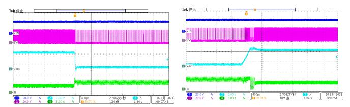
Figure 17. Over Current Protection(3A to hard short)
