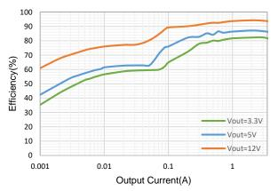
Figure 3. Efficiency vs Load Current, Vin=24V
