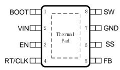
Figure 1. 8-Lead Plastic ESOP
