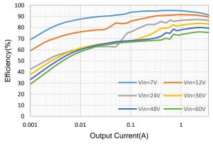
Figure 2. Efficiency vs Load Current, Vout=5V
