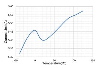
Figure 5. Current Limit VS Temperature
