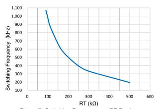
Figure 7. Switching Frequency vs RT Resistor
