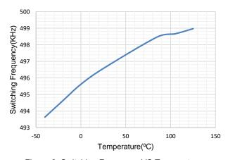
Figure 6. Switching Frequency VS Temperature
