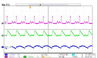
Figure 21. Output Ripple (Iload=0A)
