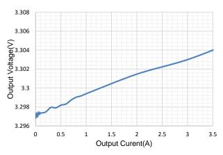
Figure 4. Load Regulation, Vin=24V, Vout=3.3V
