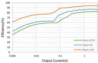
Efficiency, Vin=24V, Fsw=500KHz
