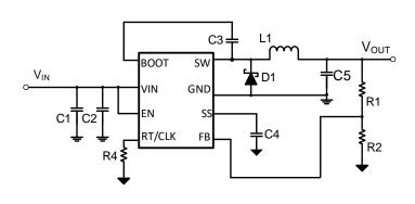
4.5V-60V, Asyncronous Buck Converter
