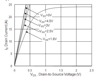
Fig.1 Typical Output Characteristics
