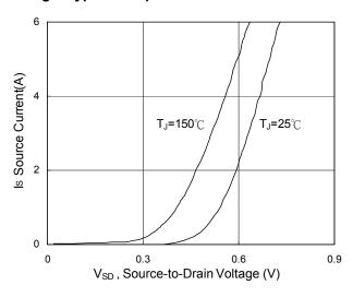
Fig.3 Forward Characteristics of reverse
