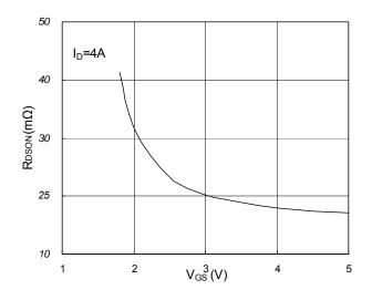
Fig.2 On-Resistance vs. Gate-Source
