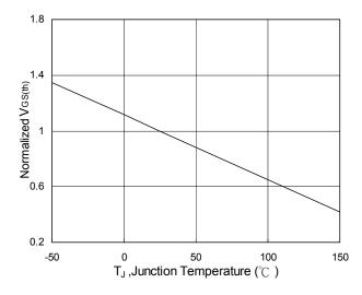
Fig.5 V<sub>GS(th)</sub> vs. T<sub>J</sub>
