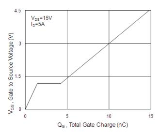
Fig.4 Gate-Charge Characteristics
