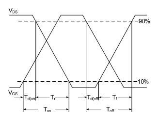
Fig.10 Switching Time Waveform
