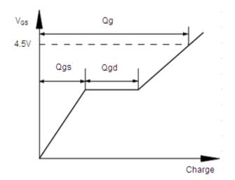
Fig.11 Gate Charge Waveform
