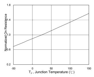
Fig.6 Normalized R<sub>DSON</sub> vs. T<sub>J</sub>
