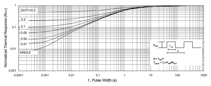
Fig.9 Normalized Maximum Transient Thermal Impedance
