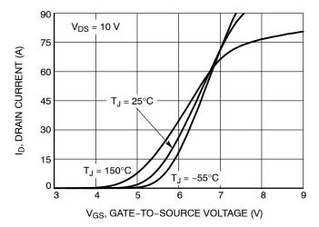
Figure 5. Transfer Characteristics
