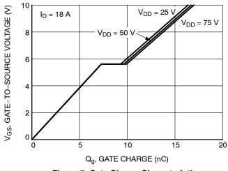
Figure 7. Gate Charge Characteristics
