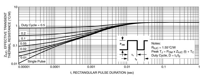
Figure 13. Transient Thermal Impedance
