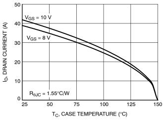
Figure 9. Drain Current vs. Case Temperature
