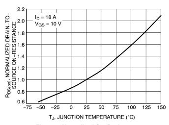
Figure 3. Normalized On–Resistance vs. Junction Temperature
