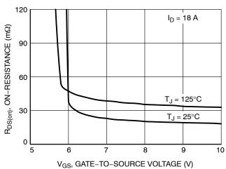
Figure 4. On-Resistance vs. Gate-to-Source Voltage
