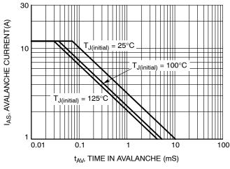
Figure 11. Unclamped Inductive Switching Capability
