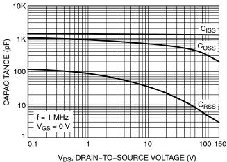
Figure 8. Capacitance vs. Drain-to-Source
