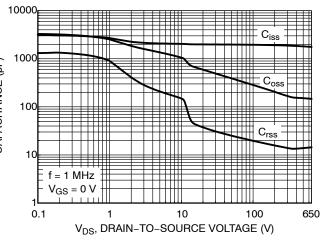
Figure 8. Capacitance vs. Drain-to-Source Voltage
