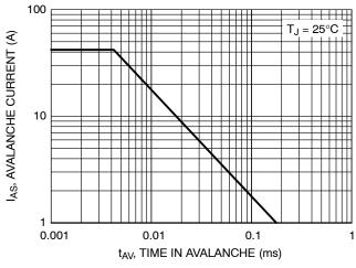
Figure 9. Unclamped Inductive Switching Capability
