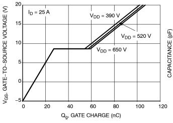
Figure 7. Gate-to-Source Voltage vs. Total Charge
