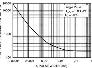
Figure 12. Single Pulse Maximum Power Dissipation
