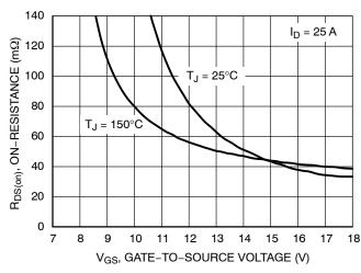
Figure 3. On–Resistance Variation with Temperature
