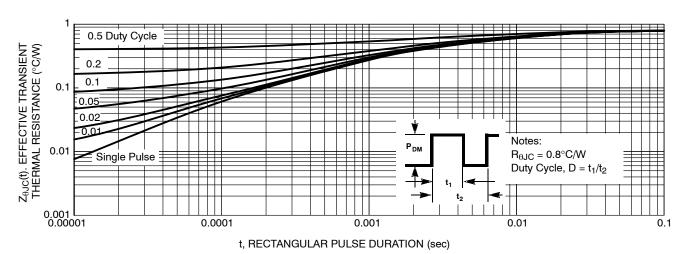
Figure 13. Junction-to-Case Thermal Response
