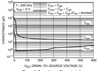
Figure 5. Capacitance Characteristics
