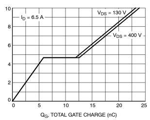
Figure 6. Gate Charge Characteristics
