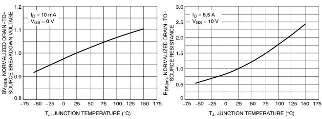
Figure 7. Breakdown Voltage Variation vs.
