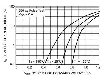
Figure 4. Diode Forward Voltage Variation vs. Source Current and Temperature
