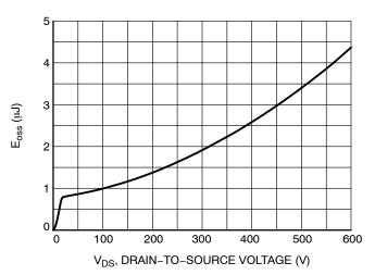
Figure 11. E<sub>oss</sub> vs. Drain-to-Source Voltage
