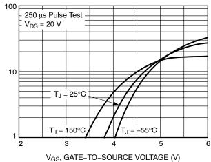
Figure 2. Transfer Characteristics
