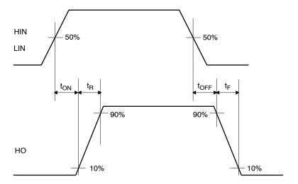
Figure 37. Switching Time Definition
