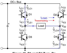
Figure 45. Q1 and Q4 Turn-On
