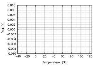
Figure 23. Low-Level Output Voltage vs. Temperature
