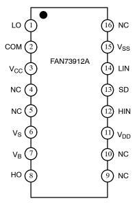
Figure 3. Pin Connections – Wide 16–SOIC (Top View)
