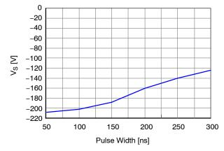
Figure 47. Negative V<sub>S</sub> Transient Characteristic
