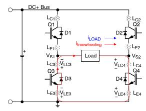
Figure 46. Q1 Turn-Off and D3 Conducting
