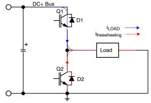
Figure 43. Half-Bridge Application Circuits
