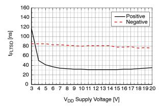
Figure 32. Shutdown Input Filtering Time vs. V<sub>DD</sub> Supply Voltage
