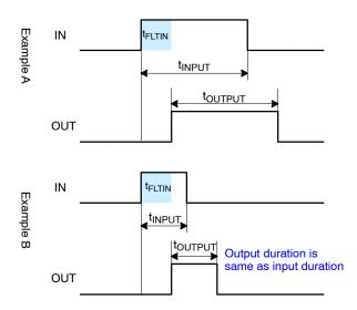
Figure 41. Input Noise Filter Definition
