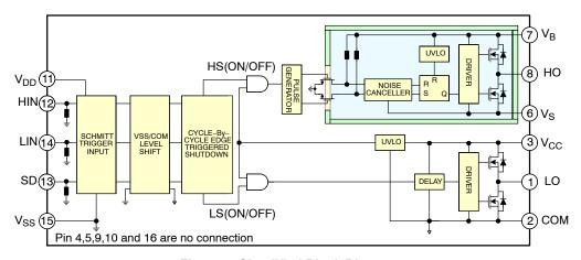
Figure 2. Simplified Block Diagram
