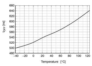
Figure 5. Turn-Off Propagation Delay vs. Temperature
