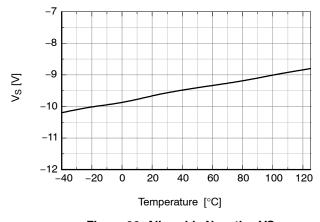
Figure 26. Allowable Negative VS vs. Temperature
