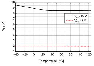
Figure 24. Logic High Input Voltage
