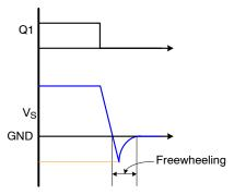
Figure 44. V<sub>S</sub> Waveforms During Q1 Turn-Off
