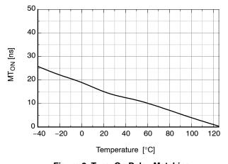
Figure 8. Turn-On Delay Matching vs. Temperature
