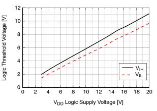
Figure 27. Input Logic (HIN&LIN) Threshold vs. V<sub>DD</sub> Supply Voltage
