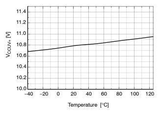
Figure 18. V<sub>CC</sub> UVLO+ vs Temperature
