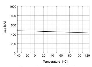
Figure 17. Operating V<sub>BS</sub> Supply Current vs. Temperature
