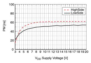
Figure 34. Output Pulse-Width Matching vs.  $V_{\rm DD}$  Supply Voltage
