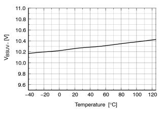
Figure 21. V<sub>BS</sub> UVLO- vs. Temperature
