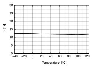
Figure 7. Turn-Off Fall Time vs. Temperature
