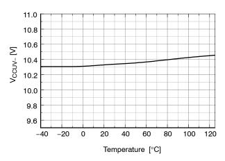
Figure 19. V<sub>CC</sub> UVLO- vs. Temperature
