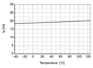
Figure 6. Turn-On Rise Time vs Temperature
