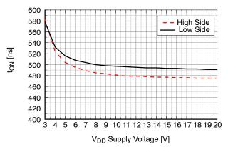
Figure 29. Turn-On Propagation Delay vs. V<sub>DD</sub> Supply Voltage
