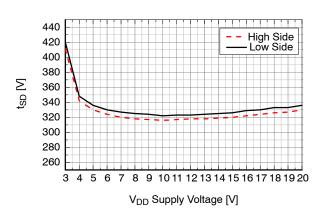
Figure 33. Shutdown Propagation Delay vs. V<sub>DD</sub> Supply Voltage
