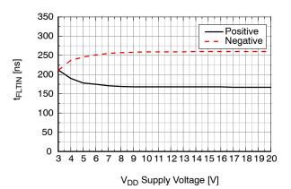
Figure 31. Logic Input Filtering Time vs. V<sub>DD</sub> Supply Voltage
