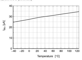
Figure 11. Logic Input High Bias Current vs. Temperature
