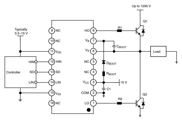
Figure 1. Application Schematic - Adjustable Option
