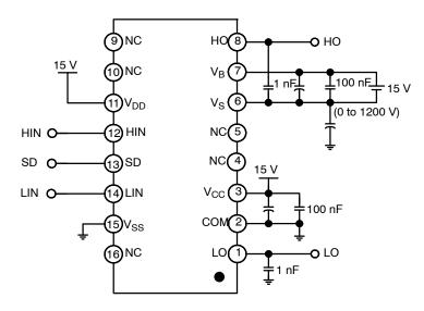
Figure 35. Switching Time Test Circuit
