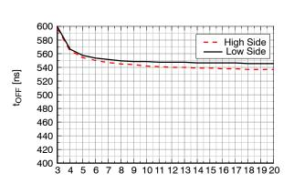
Figure 30. Turn-Off Propagation Delay vs. V<sub>DD</sub> Supply Voltage
