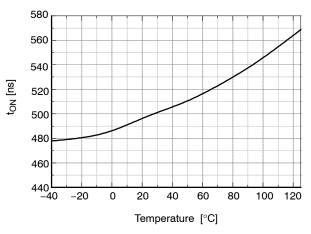
Figure 4. Turn-On Propagation Delay vs. Temperature
