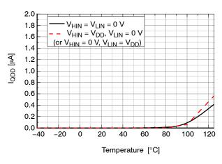
Figure 13. Quiescent V<sub>DD</sub> Supply Current vs. Temperature
