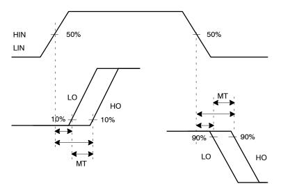
Figure 39. Delay Matching Waveform Definitions
