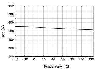
Figure 15. Operating  $V_{CC}$  Supply Current
