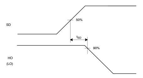
Figure 38. Shutdown Waveform Definition
