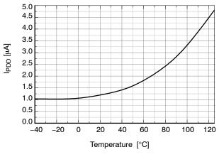
Figure 16. Operating V<sub>DD</sub> Supply Current
