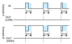
Figure 42. Noise Rejecting Input Filter Definition
