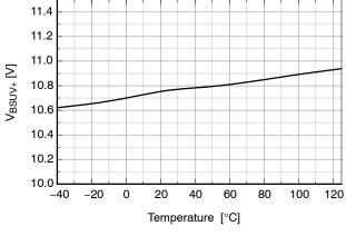
Figure 20. V<sub>BS</sub> UVLO+ vs. Temperature
