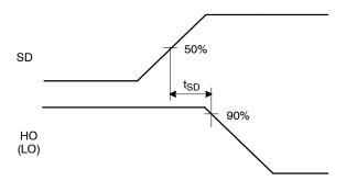
Figure 40. Output Shutdown Timing Waveform
