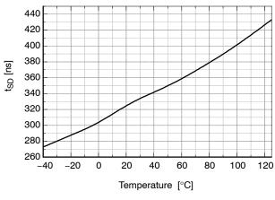
Figure 10. Shutdown Propagation Delay vs. Temperature
