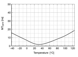
Figure 9. Turn-Off Delay Matching vs. Temperature
