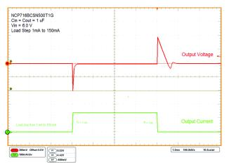
Figure 17. Load Transient Response
