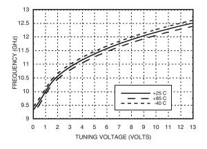
Divide-by-16 Frequency vs. Tuning Voltage, Vcc= +5V
