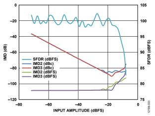
Figure 34. Two Tone SFDR/IMD vs. Input Amplitude, for f<sub>IN</sub> = 184 MHz and 187 MHz, Dither Enabled, Register 0x22A = 0x01
