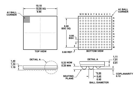
\*COMPLIANT WITH JEDEC STANDARDS MO-275-EEAA-1 WITH THE EXCEPTION TO BALL DIAMETER.
