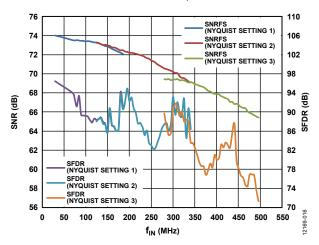
Figure 28. Single Tone SNR/SFDR vs. Input Frequency ( $f_{IN}$ ), Amplitude = -1 dBFS,  $V_{REF} = 1.0 \text{ V}$
