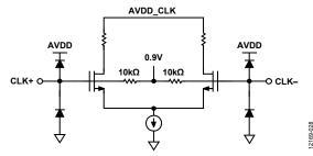
Figure 43. Equivalent Clock Circuit
