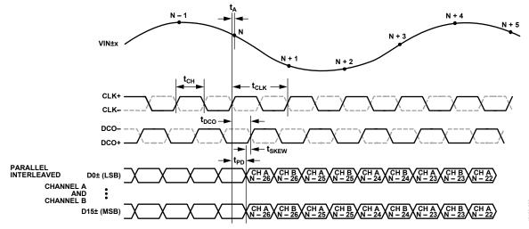
Figure 2. LVDS Data Output Timing
