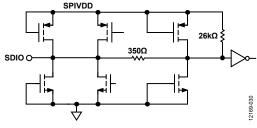
Figure 45. Equivalent SDIO Circuit
