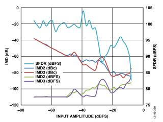
Figure 31. Two Tone SFDR/IMD vs. Input Amplitude, for  $f_{\rm IN}$  = 184 MHz and 187 MHz, Dither Disabled, Register 0x22A = 0x01
