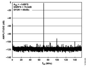
Figure 6. Single Tone Fast Fourier Transform (FFT) with  $f_{\text{IN}}$  = 70.1 MHz (NSD = -156.7 dBFS/Hz)
