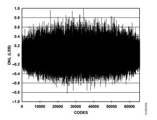
Figure 37. DNL with Dither Off,  $f_{IN} = 30 \text{ MHz}$
