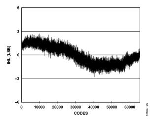
Figure 41. INL with Dither On,  $f_{IN} = 30 \text{ MHz}$
