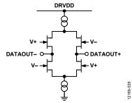
Figure 44. Equivalent LVDS Output Circuit (DCO $\pm$ , OR $\pm$ , and D0 $\pm$  to D15 $\pm$ )
