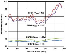
Figure 36. Encode Rate Sweep,  $f_{\rm IN}$  = 90.1 MHz at -7 dBFS,  $V_{\rm REF}$  = 1.25 V and 1.0 V
