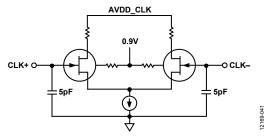
Figure 59. Simplified Equivalent Clock Input Circuit
