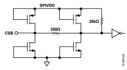
Figure 48. Equivalent CSB Input Circuit
