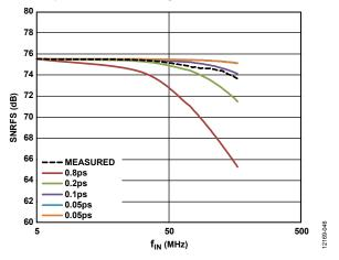
Figure 64. SNRFS vs. Input Frequency and Jitter
