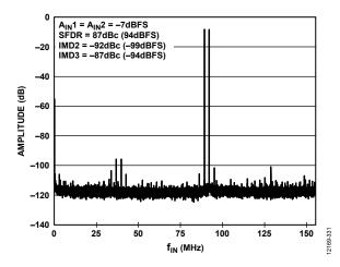
Figure 32. Two Tone FFT with  $f_{\rm IN}$  = 89.1 MHz and 92.1 MHz, VREF = 1.25 V
