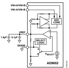
Figure 57. Internal Reference Configuration
