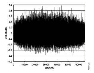
Figure 38. DNL with Dither On,  $f_{IN} = 30 \text{ MHz}$
