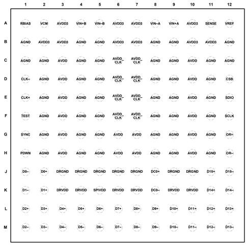
Figure 5. Pin Configuration
