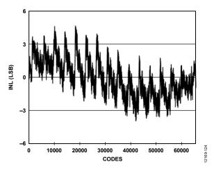
Figure 40. INL with Dither Off,  $f_{IN} = 30 \text{ MHz}$
