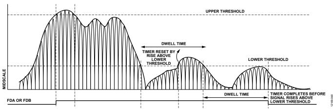
Figure 66. Threshold Settings for FDA and FDB Signals
