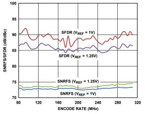
Figure 39. Encode Rate Sweep,  $f_{\rm IN}$  = 90.1 MHz at -1 dBFS,  $V_{\rm REF}$  = 1.25 V and 1.0 V
