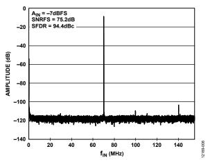
Figure 10. Single Tone FFT with  $f_{\rm IN}$  = 70.1 MHz at -7 dBFS with Dither (NSD = -157.1 dBFS/Hz)
