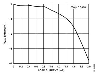
Figure 58. Reference Voltage Error vs. Load Current
