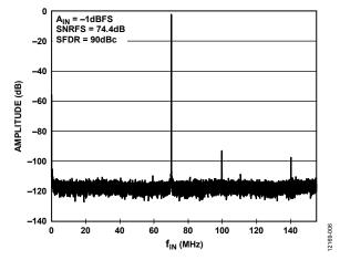
Figure 9. Single Tone FFT with  $f_{\rm IN}$  = 70.1 MHz with Dither (NSD = -156.3 dBFS/Hz)
