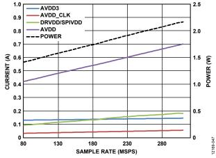
Figure 65. Power and Current vs. Sample Rate
