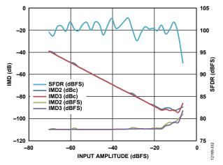
Figure 33. Two Tone SFDR/IMD vs. Input Amplitude, for  $f_{\rm IN}$  = 70.1 MHz and 72.1 MHz, Dither Enabled
