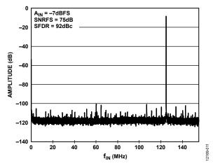
Figure 12. Single Tone FFT with  $f_{\rm IN}=185$  MHz at -7 dBFS (NSD = -156.9 dBFS/Hz), Register 0x22A = 0x01
