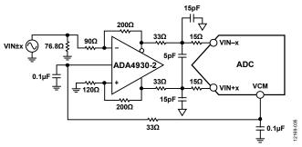
Figure 53. Differential Input Configuration Using the ADA4930-2
