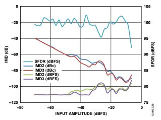
Figure 30. Two Tone SFDR/Intermodulation Distortion (IMD) vs. Input Amplitude, for  $f_{\rm IN}=70.1$  MHz and 72.1 MHz, Dither Disabled
