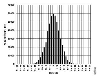
Figure 35. Grounded Input Histogram
