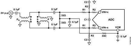
Figure 56. Differential Double Balun Input Configuration
