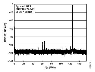
Figure 11. Single Tone FFT with  $f_{\rm IN}$  = 185 MHz at -1 dBFS with Dither (NSD = -154.9 dBFS/Hz), Register 0x22A = 0x01
