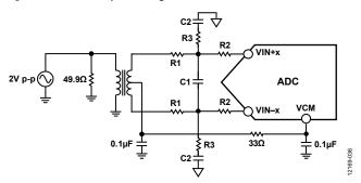
Figure 54. Differential Transformer-Coupled Configuration
