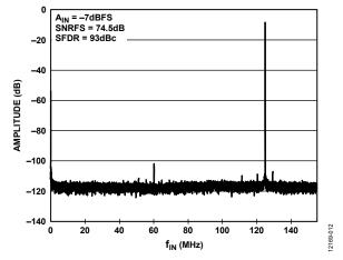
Figure 15. Single Tone FFT with  $f_{\rm IN}$  = 185 MHz at -7 dBFS with Dither (NSD = -156.4 dBFS/Hz), Register 0x22A = 0x01
