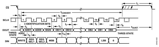
Figure 2. Serial Interface Timing Diagram
