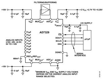
Figure 34. Typical Connection Diagram, Single-Ended Mode
