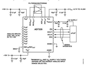
Figure 35. Typical Connection Diagram, Differential Mode
