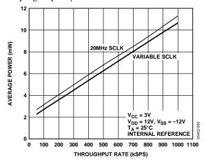
Figure 55. Power vs. Throughput Rate with 3 VVcc
