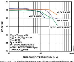
Figure 13. SINAD vs. Analog Input Frequency for True Differential Mode at 5 V Vcc
