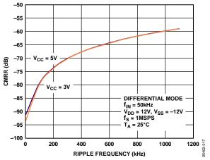
Figure 17. CMRR vs. Common-Mode Ripple Frequency
