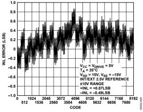
Figure 9. Typical INL for Single-Ended Mode
