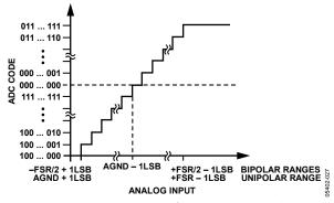
Figure 28. Twos Complement Transfer Characteristic, Bipolar Ranges
