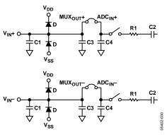
Figure 31. Equivalent Analog Input Circuit, Differential Mode
