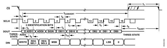
Figure 57. Serial Interface Timing Diagram (Control Register Write)
