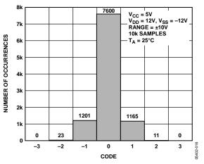
Figure 16. Histogram of Codes, Single-Ended Mode
