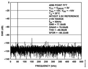
Figure 4. FFT for True Differential Mode
