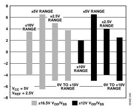
Figure 43. Pseudo Differential Input Range with  $V_{CC} = 5 \text{ V}$
