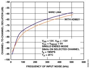
Figure 14. Channel-to-Channel Isolation with and Without AD8021 Between the MUX<sub>OUT</sub>+ and ADC<sub>IN</sub>+ Pins
