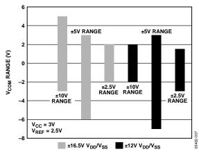
Figure 40. Common-Mode Range for  $V_{CC} = 3 \text{ V}$  and  $REF_{IN}/REF_{OUT} = 2.5 \text{ V}$
