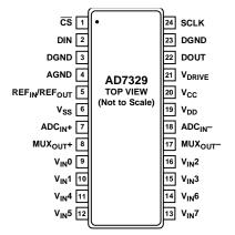
Figure 3. Pin Configuration
