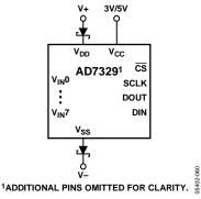
Figure 60. Schottky Diode Connection
