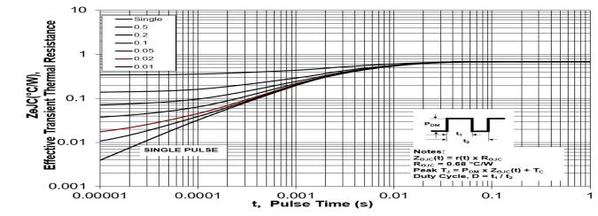
Figure 13. Junction-to-Ambient Thermal Response
