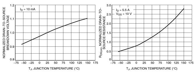
Figure 7. Normalized BV<sub>DSS</sub> vs. Temperature
