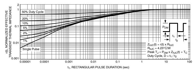
Figure 11. Transient Thermal Impedance
