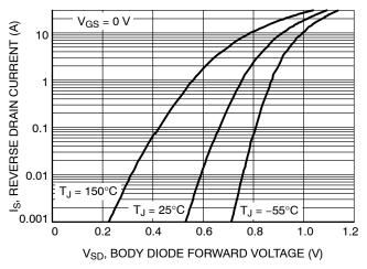
Figure 4. Diode Forward Voltage vs. Current
