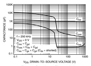
Figure 5. Capacitance Characteristics
