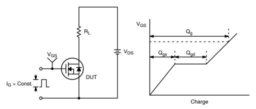
Figure 12. Gate Charge Test Circuit & Waveform
