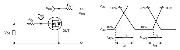
Figure 13. Resistive Switching Test Circuit & Waveforms
