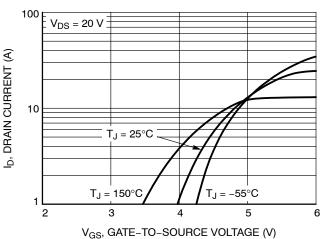
Figure 2. Transfer Characteristics
