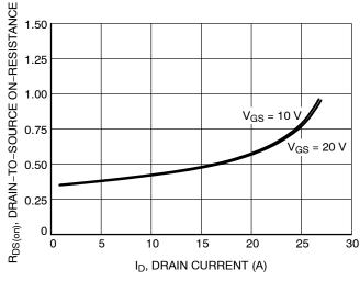
Figure 3. On Resistance vs. Drain Current
