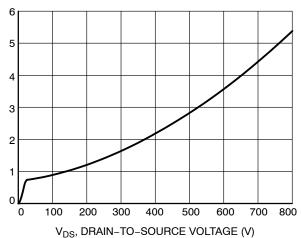
Figure 10. E<sub>oss</sub> vs. Drain-to-Source Voltage
