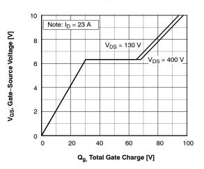
Figure 6. Gate Charge Characteristics
