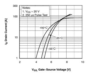
Figure 2. Transfer Characteristics
