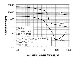
Figure 5. Capacitance Characteristics
