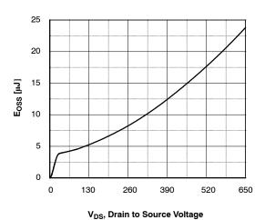
Figure 11. E<sub>oss</sub> vs. Drain to Source Voltage
