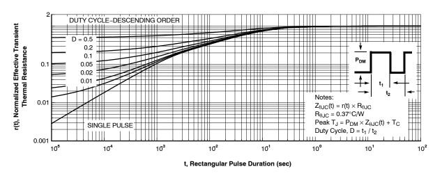
Figure 12. Transient Thermal Response Curve
