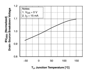
Figure 7. Breakdown Voltage Variation vs. Temperature
