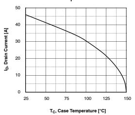
Figure 10. Maximum Drain Current vs.
