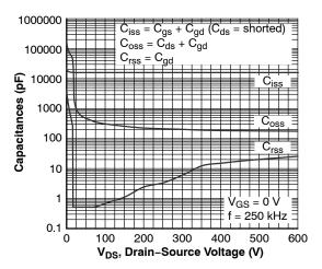
Figure 5. Capacitance Characteristics
