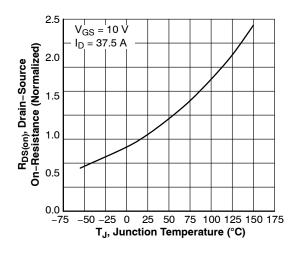
Figure 8. On–Resistance Variation vs. Temperature
