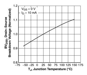
Figure 7. Breakdown Voltage Variation vs. Temperature
