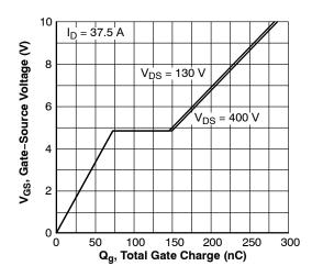
Figure 6. Gate Charge Characteristics
