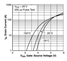
Figure 2. Transfer Characteristics
