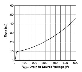
Figure 11.  $E_{\mbox{\scriptsize OSS}}$  vs. Drain to Source Voltage
