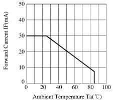
Fig.6 Forward Current Derating Curve
