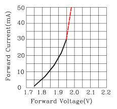
Fig.2 Forward Current vs.Forward Voltage
