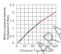
Fig.4 Relative Luminous Intensity vs.Forward Current
