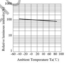
Fig.5 Luminous Intensity vs. Ambient Temperature
