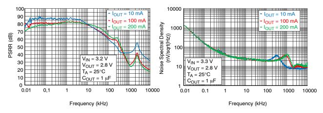
Figure 14. Power Supply Rejection Ration for  $V_{OUT} = 2.8 \text{ V}$ ,  $C_{OUT} = 1 \mu\text{F}$
