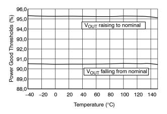
Figure 12. Power Good Threshold vs. Temperature
