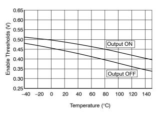
Figure 11. Enable Thresholds vs Temperature
