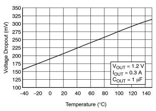
Figure 5. Dropout Voltage vs. Temperature –  $V_{OUT} = 1.2 \text{ V}$
