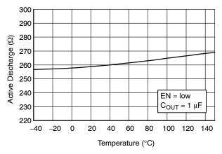
Figure 13. Active Discharge Resistance vs. Temperature
