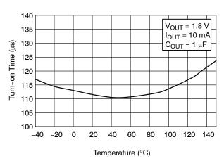
Figure 9. Turn-on Time vs. Temperature
