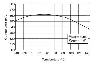
Figure 10. Current Limit vs. Temperature
