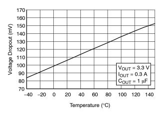
Figure 7. Dropout Voltage vs. Temperature –  $V_{OUT} = 3.3 \text{ V}$
