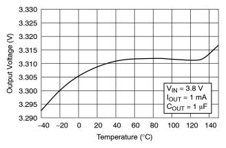
Figure 4. Output Voltage vs. Temperature –  $V_{OUT} = 3.3 \text{ V}$
