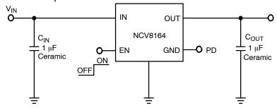
Figure 1. Typical Application Schematics
