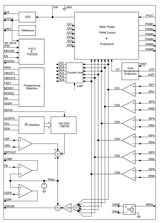
Figure 5. Functional Block Diagram
