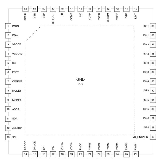
Figure 1. Pin Configuration
