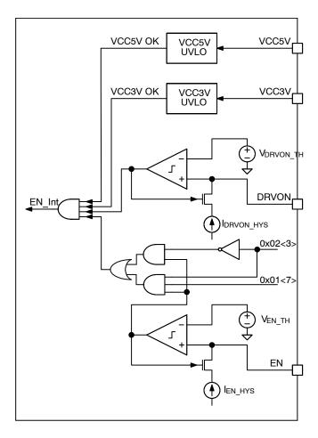
Figure 9. Enable, DRVON and UVLO
