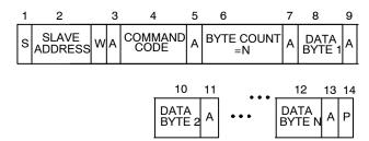
Figure 25. Block Write to a Register
