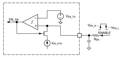
Figure 10. Enable and Hysteresis Programming
