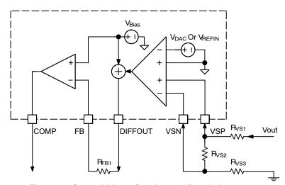
Figure 14. Output Voltage Sensing and Regulation
