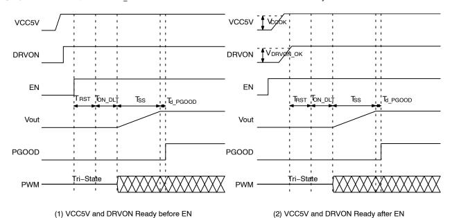
Figure 6. Timing Diagrams of Power Up Sequence
