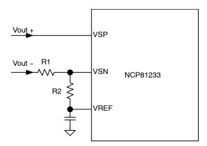
Figure 15. Adding Offset Voltage in Output
