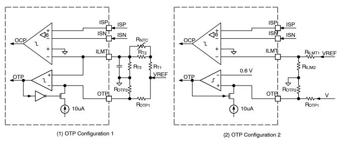
Figure 18. Over-Current Protection and Over-Temperature Protection
