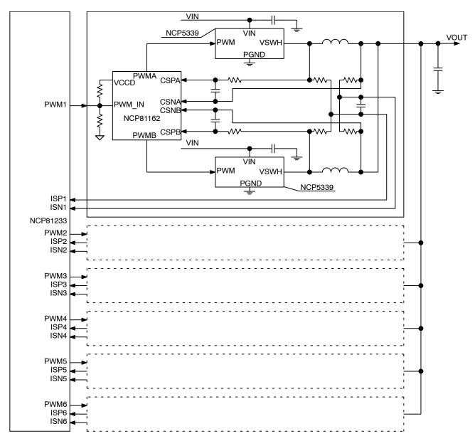
Figure 4. Application Circuit with Phase Doublers
