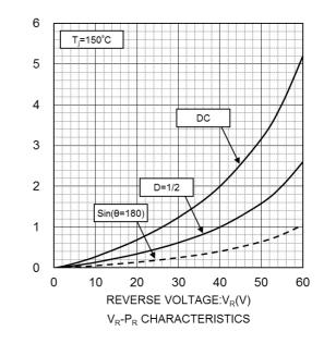
REVERSE POWER DISSIPATION:P<sub>R</sub>(mW)
