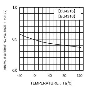
Fig.12 Operating Limit Voltage
