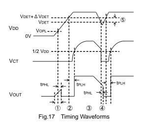
(1) When the power supply is turned on, the output is unstable from after over the operating limit voltage (VOPL) until tPHL. Therefore, it is possible that the reset signal is not outputted when the rise time of VDD is faster than tPHL.
