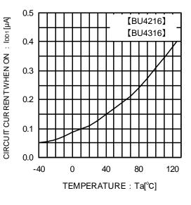
Fig.10 Circuit Current when ON
