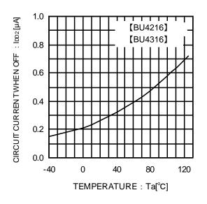
Fig.11 Circuit Current when OFF
