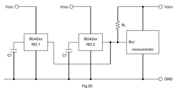
To reset the microcontroller when many independent power supplies are used in the system, OR connect an open drain output type (BU42xx series) to the microcontroller's input with pull-up resistor to the supply voltage of the microcontroller (V<sub>DD3</sub>) as shown in Fig. 20. By pulling-up to V<sub>DD3</sub>, output "High" voltage of micro-controller power supply is possible.
