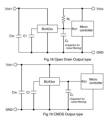
Application examples of BU42xx series (Open Drain output type) and BU43xx series (CMOS output type) are shown below.
