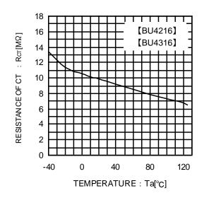
Fig.13 CT Terminal Circuit Resistance
