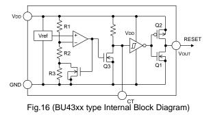
C<sub>T</sub> pin Threshold Voltage(P.3 VCTH refer.)
