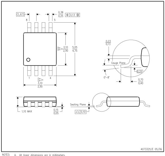
A. All linear dimensions are in millimeters.
