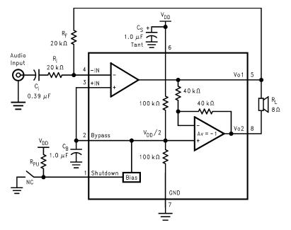
Figure 3. Typical Audio Amplifier Application Circuit
