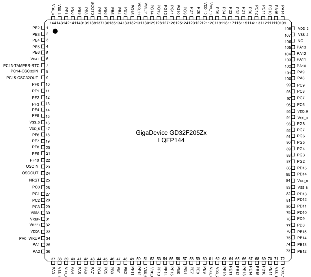
Figure 2-2. GD32F205Zx LQFP144 pinouts
