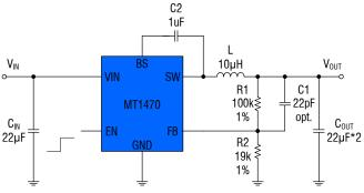
Figure 1. Basic Application Circuit
