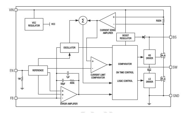
Figure 2. MT1470 Block Diagram
