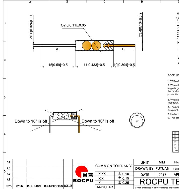
**ROCPU** Product features Voltage: < 5V Current: < 20mA Conduction time: 2ms Closed circuit resistance: < 100hm Open circuit resistance: > 20m ohm High temperature resistance:120 ℃/260 ℃ Terminal tension: 1000gf / min Humidity: 25~95%RH Working lifespan:20,000 cycles Error rate:1%
