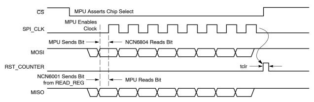
Figure 11. Basic SPI Timings and Protocol
