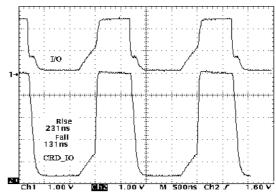
Figure 9. Typical I/O rise & fall time (CRD\_IOA or B/ C<sub>out</sub> > 30 pF and open-drain)
