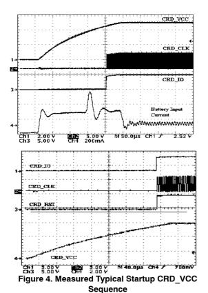
At powerup, the CRD\_VCCA/B turn-on time depends upon the current capability of the DC/DC converter associated with the external inductor L and the reservoir capacitor connected across CRD\_VCCA or B and GROUND. During this sequence, the average input current is 300 mA typical (see Figure 4), assuming the system is fully loaded during the start up.
