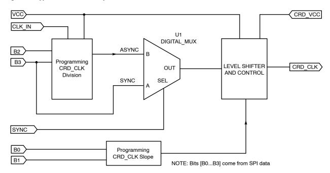
Figure 23. Basic Clock Divider and Level Shifter
