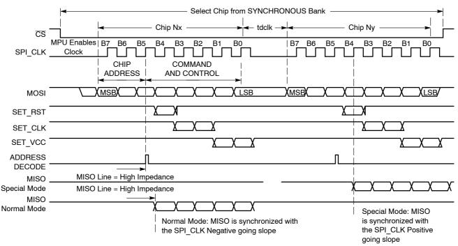
Figure 13. Basic Multi Command SPI Bytes
