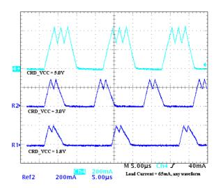
**Figure 19. Typical Inductor Current**
