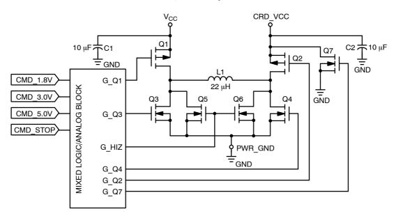
Figure 16. Basic DC/DC Converter
