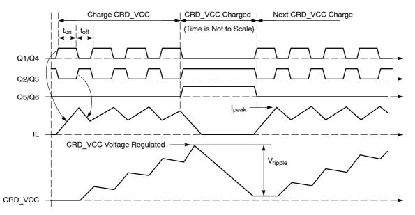
Figure 17. Theoretical DC/DC Operating Waveforms
