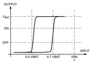
Figure 24. Typical Schmitt Trigger Characteristic
