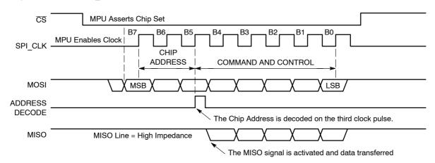
Figure 12. Chip Address Decoding Protocol and MISO Sequence
