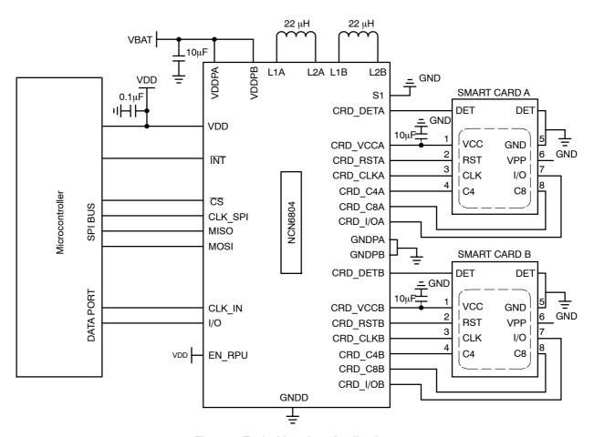
Figure 1. Typical Interface Application
