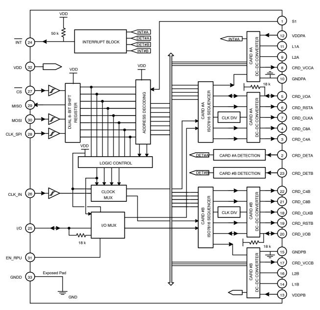
Figure 2. NCN6804 Block Diagram
