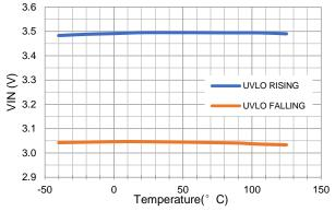
Figure 2. VIN UVLO vs Temperature
