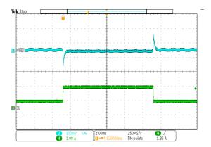
Figure 16. Load Transient (Vout=5V, lout=0.5A to 1.5A, SR=250mA/us)
