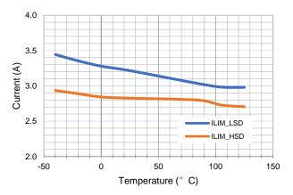
Figure 6. Peak Current Limit vs Temperature
