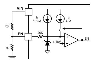
Figure 7. Adjustable VIN UVLO
