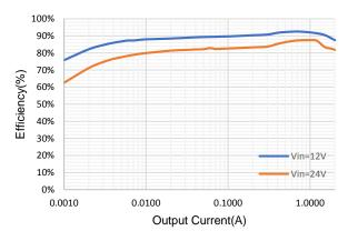
Figure 1. Efficiency, Vout=3.3V
