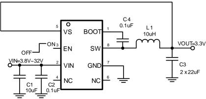
Figure 10. 12V Input, 3.3V/2A Output
