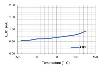
Figure 3. Shut down Current vs Temperature
