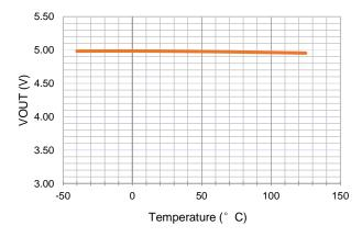
Figure 5. Output Voltage vs Temperature
