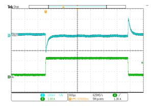
Figure 15. Load Transient (Vout=5V, lout=0.2A to 1.8A, SR=250mA/us)
