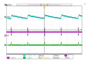
Figure 12. SW node Waveform and Output Ripple, lout=10mA
