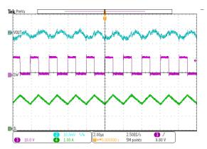
Figure 11. SW node waveform and Output Ripple, lout=2A
