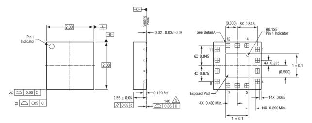
Figure 4. FM3418C 14-Pin QFN Package Dimensions
