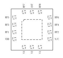
Figure 2. FM3418C Pinout - 14-Pin QFN (Top View)
