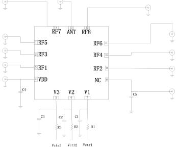
Figure 3. FM3418C Application Schematic
