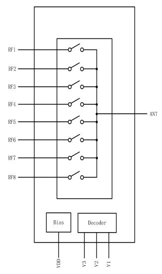
Figure 1. FM3418C Block Diagram
