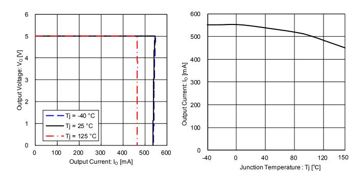
Figure 7. Output Voltage vs. Output Current (Over Current Protection)
