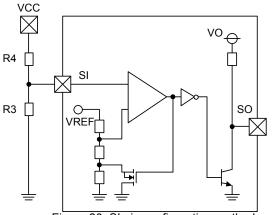
Figure 20. SI pin configuration method
