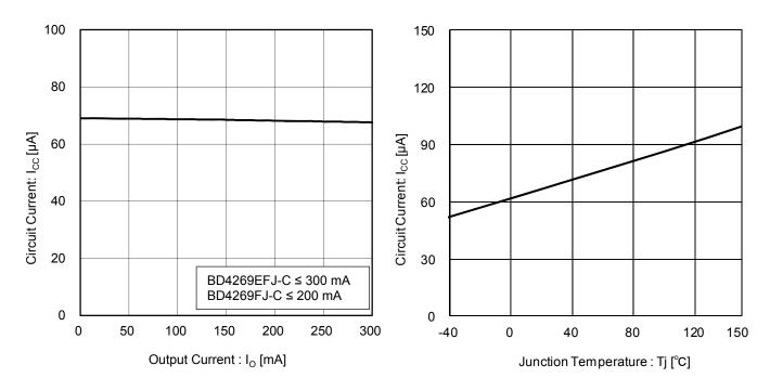
Figure 5. Circuit Current vs. Output Current
