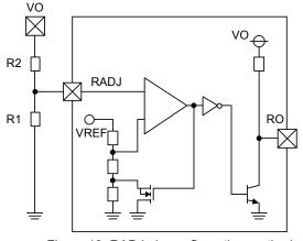
Figure 19. RADJ pin configuration method
