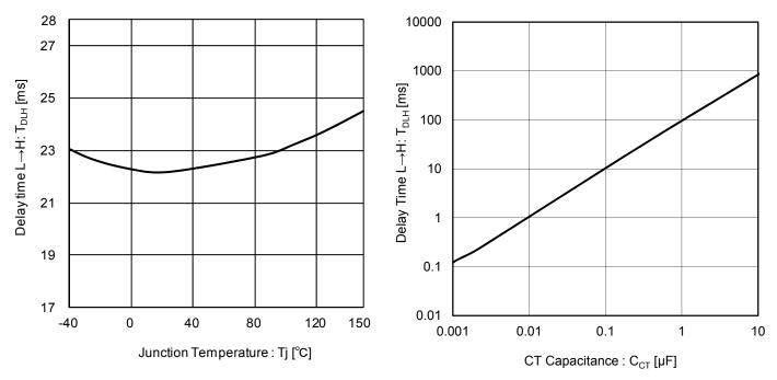
Figure 13. Delay Time L $\rightarrow$ H vs. Junction Temperature (C<sub>CT</sub> = 0.22  $\mu$ F)
