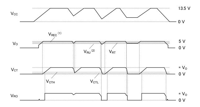
$<sup>^{(1)}</sup>$  V\_{REC} = V\_{RT} + V\_{RHY}  $^{(2)}$  V\_{RU} = 2 to 3.5 V  $^{(3)}$  When RADJ is used, V\_{RT} = V\_RTADJ, V\_{REC} = V\_{RTADJ} + V\_RHY
