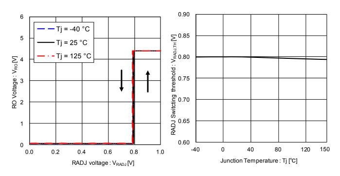
Figure 15. RO Voltage vs. RADJ Voltage
