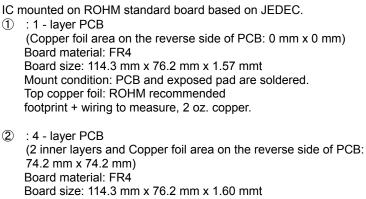
Mount condition: PCB and exposed pad are soldered.
