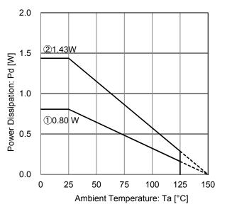
Figure 21. SOP-J8 Package Data (Reference Data)
