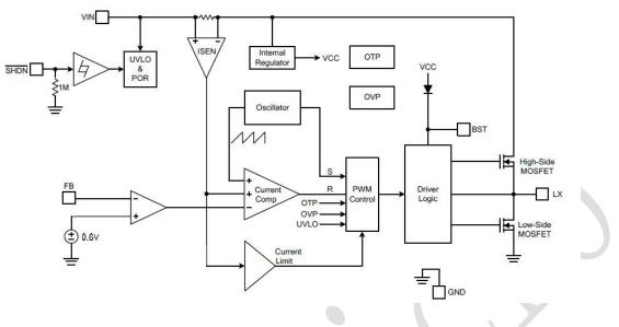
Figure 2. TMI3280 Block Diagram
