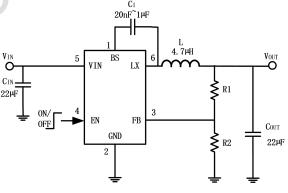
Figure 1. Basic Application Circuit
