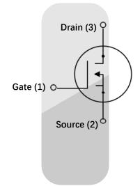
These devices are N-channel 650 V Power GaN HEMTs based on proprietary E-mode GaN on silicon technology. The resulting product has extremely low on state resistance, very low input capacitance and zero reverse recovery charge making it especially suitable for applications which require superior power density, ultra-high switching frequency and outstanding efficiency.
