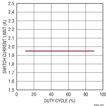
Switch Current Limit vs Duty Cycle
