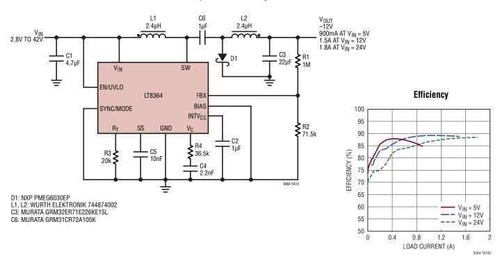
2MHz, 2.8V to 42V Input, -12V Inverting Converter
