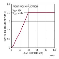
Figure 1. Burst Frequency vs Load Current
