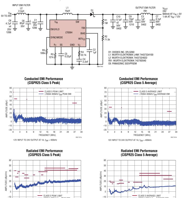
Low IQ, Low EMI, 400kHz, 24V Boost Converter with SSFM
