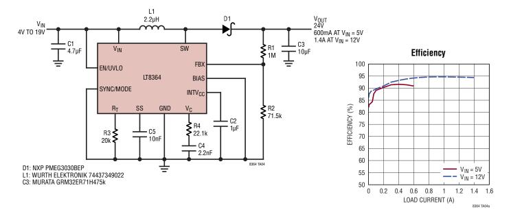
2MHz, 2.8V to 6V Input, 48V Boost Converter in DCM
