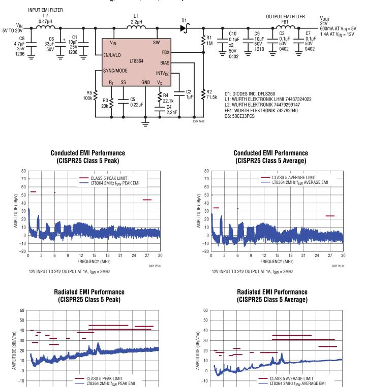
Low IQ, Low EMI, 2MHz, 24V Output Boost Converter with SSFM
