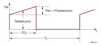
Figure 7. The Switch Current Waveform of the SEPIC Converter
