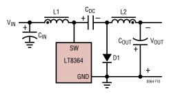
Figure 8. A Simplified Inverting Converter
