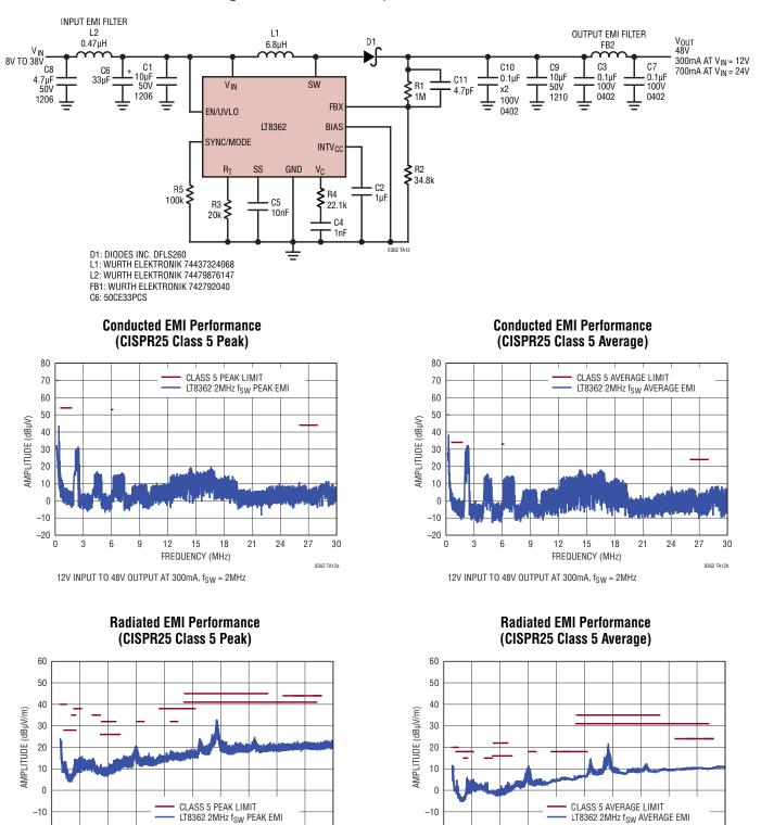
Low  $I_Q$ , Low EMI, 2MHz, 48V Output Boost Converter with SSFM
