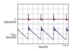
Figure 2. Burst Mode Operation
