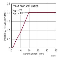
Figure 1. Burst Frequency vs Load Current
