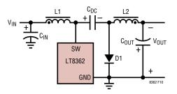
Figure 8. A Simplified Inverting Converter
