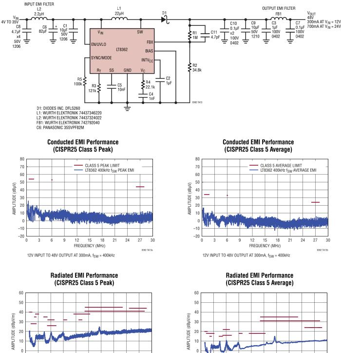
Low IQ, Low EMI, 400kHz, 48V Boost Converter with SSFM
