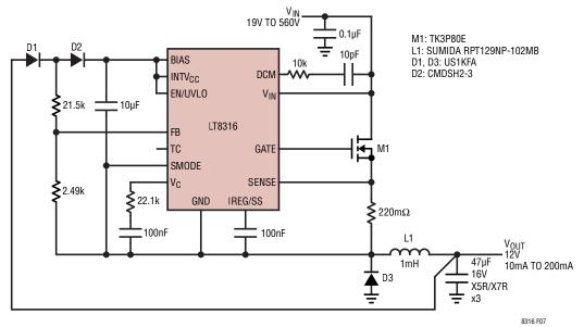
Figure 7. Ultra-Wide Input Range Non-Isolated 12V Buck Converter
