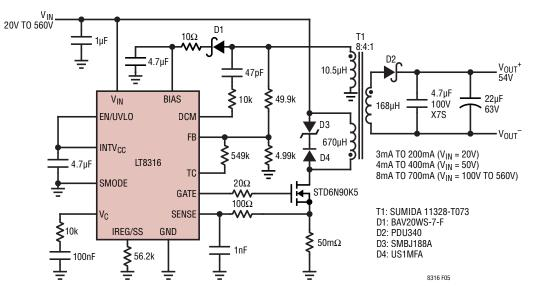
Figure 5. 94% Efficient Isolated 54V Supply
