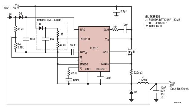
Figure 9. Nonisolated 24V Buck Converter with Optional Undervoltage Lockout
