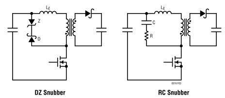
Figure 3. Snubber Circuits
