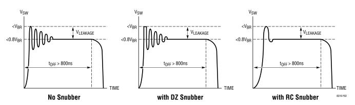
Figure 2. Maximum Voltages for SW Pin Flyback Waveform
