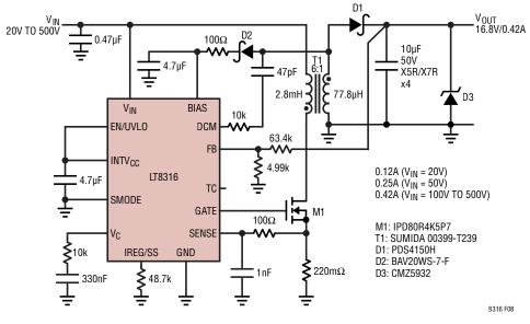
Figure 8. Non-Isolated 16.8V Gate Drive Supply
