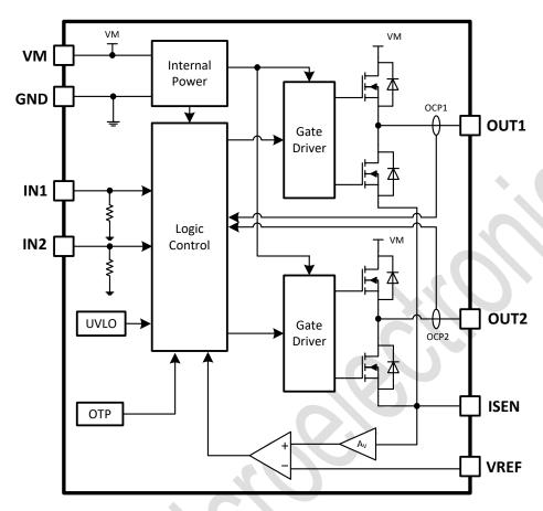
Figure 2. TMI8870/B Block Diagram
