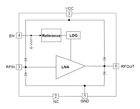
Figure 1. BCT5007 FUNCTION BLOCK DIAGRAM
