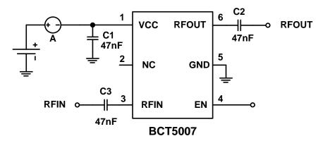
Figure 10. BCT5007 DC Test diagram
