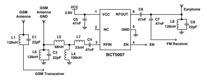
Figure 2. BCT5007 typical application circuit
