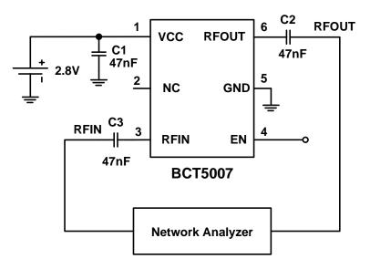
Figure 11. BCT5007 S-parameter measurement Diagram
