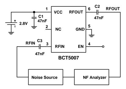
Figure 12. BCT5007 Noise Figure Measurement Diagram
