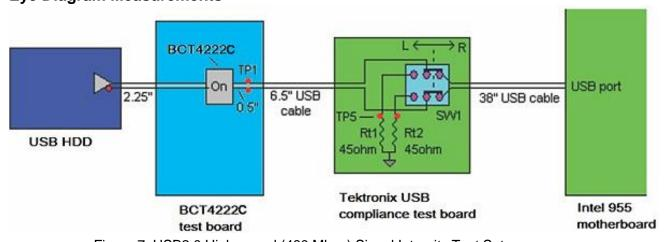
Figure 7: USB2.0 High-speed (480 Mbps) Signal Integrity Test Setup
