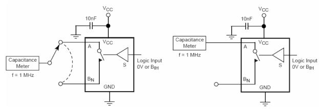
Figure 3. Channel ON/OFF Capacitance
