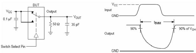
Figure 1. t<sub>BBM</sub> (Time Break-Before-Make)
