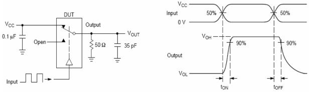
Figure 2. t<sub>ON</sub> / t<sub>OFF</sub>
