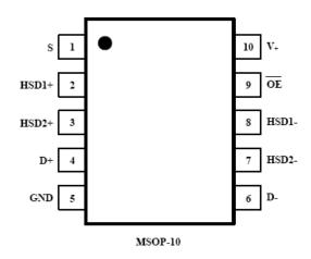
Figure 1. Pin Connections (BCT4222C Top View)
