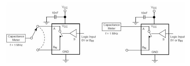
Figure 5. Channel ON/OFF Capacitance
