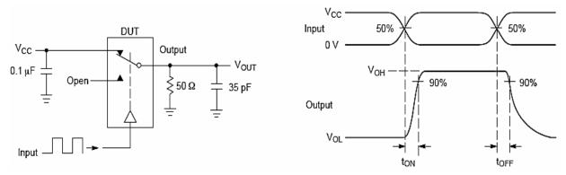
Figure 1. t<sub>ON/OFF</sub>
