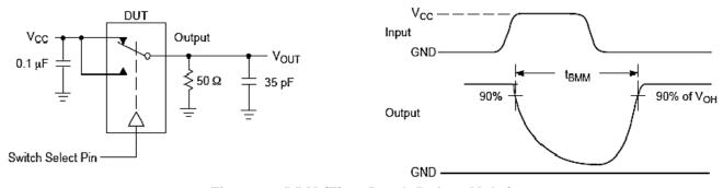
Figure 2. tBBM (Time Break-Before-Make)
