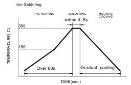
Iron Soldering times: 1 times max.
