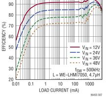
LT8645S Low Load Efficiency at 5V<sub>OUT</sub>
