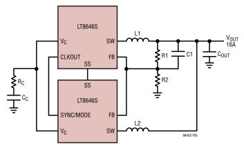
Figure 5. Paralleling Two LT8646S
