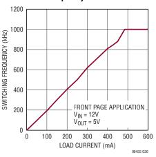
Minimum Load to Full Frequency (Pulse-Skipping Mode)
