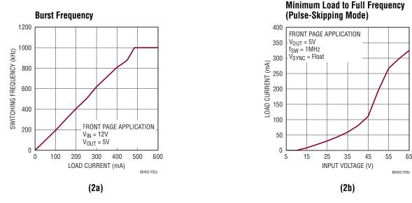
Figure 2. SW Frequency vs Load Information in Burst Mode Operation (2a) and Pulse-Skipping Mode (2b)
