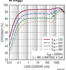
LT8646S Low Load Efficiency at 5V<sub>OUT</sub>
