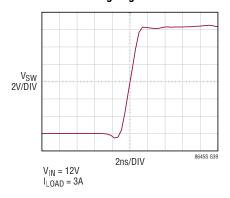
Switching Waveforms, Burst Mode Operation
