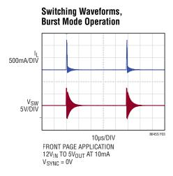
Figure 3. Burst Mode Operation
