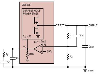
Figure 4. Model for Loop Response
