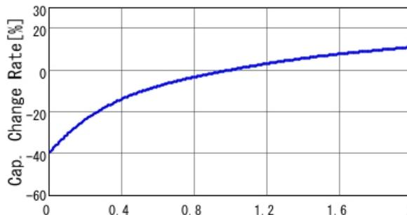
■ GRT155C8YA224KE01 C-AC Voltage capchange, DC0V, 25.0d
