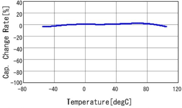
■ GRT155C8YA224KE01 C-Temp. capchange, DC0.0V, AC1.0Vrm
