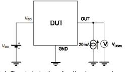
Note 1 - The output saturation voltage VDSon is measeured at VDD=3.8V and VDD=24V
