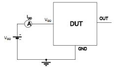
Note 1 - The supply current IDD represents the static supply current. OUT is left open during measurement
