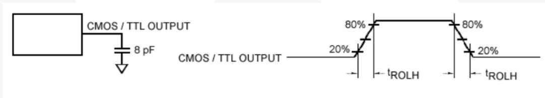
Figure 9. Receiver LVTTTL/CMOS Output Load and Transition Times
