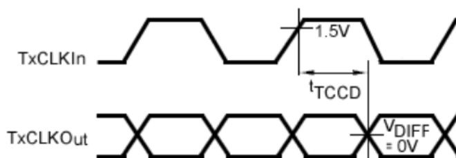
Figure 13. Transmitter Clock-In to Clock-Out Delay (Rising Edge Strobe)
