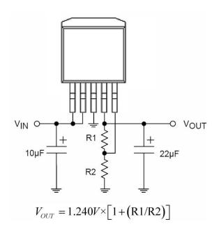
Fig. Adjustable Regulator with Resistors
