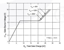
Figure 6. Gate Charge Characteristics
