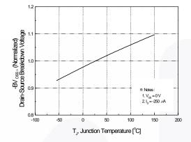
Figure 7. Breakdown Voltage Variation vs. Temperature
