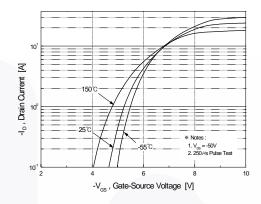
Figure 2. Transfer Characteristics
