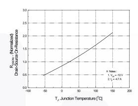
Figure 8. On-Resistance Variation vs. Temperature
