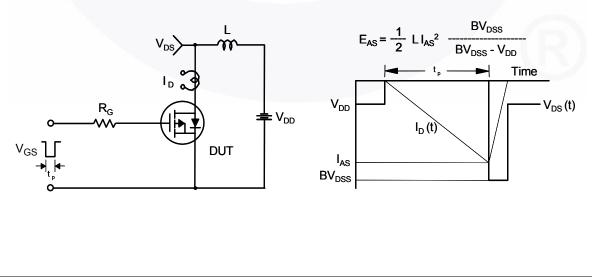
Figure 15. Peak Diode Recovery dv/dt Test Circuit & Waveforms DUT I<sub>SD</sub> o Driver Compliment of DUT ‡ VDD (N-Channel)  $\prod V_{GS}$ • dv/dt controlled by R<sub>G</sub>  $\bullet$  I<sub>SD</sub> controlled by pulse period Gate Pulse Width  $V_{GS}$ Gate Pulse Period 10V (Driver) **Body Diode Reverse Current** I<sub>SD</sub> (DUT) di/dt  $I_{\text{FM}}$  , Body Diode Forward Current  $V_{DS}$  $V_{SD}$ (DUT) Body Diode Forward Voltage Drop Body Diode Recovery dv/dt
