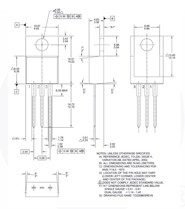
Figure 16. TO-220, Molded, 3Lead, Jedec Variation AB
