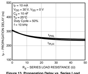
Figure 13. Propagation Delay vs. Series Load Resistance
