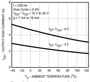
Figure 3. Output High Current vs. Ambient Temperature
