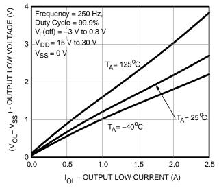
Figure 4. Output Low Voltage vs. Output Low Current
