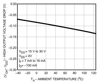
Figure 2. Output High Voltage Drop vs. Ambient Temperature
