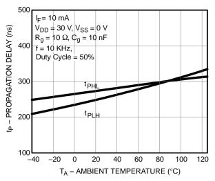
Figure 12. Propagation Delay vs. Ambient Temperature
