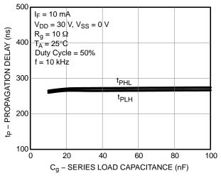
Figure 14. Propagation Delay vs. Load Capacitance
