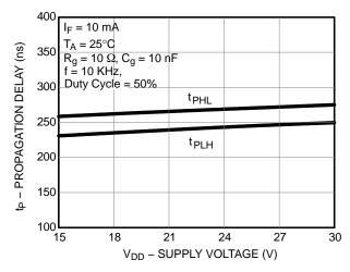
Figure 10. Propagation Delay vs. Supply Voltage
