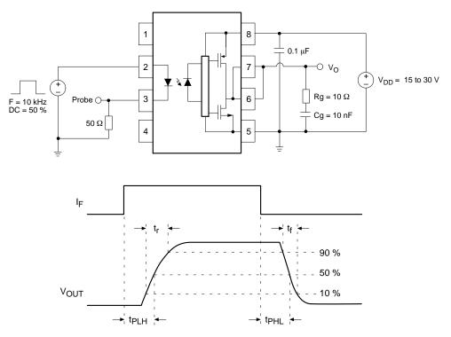
Figure 27. t<sub>PHL</sub>, t<sub>PLH</sub>, t<sub>R</sub> and t<sub>F</sub> Test Circuit and Waveforms
